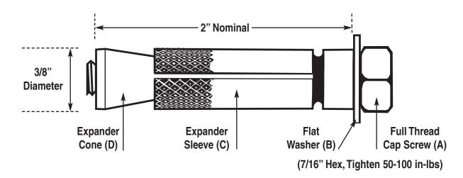
Torque Activated: 50 – 100 in – Ib = Hex Head Finish – Low Profile = Bolt Head Provides Inspection Source
